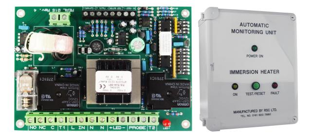
Connect all field wiring to the appropriate terminals within the unit. This should be carried out by a qualified electrician, and in accordance with bs7671 17th edition regs.
